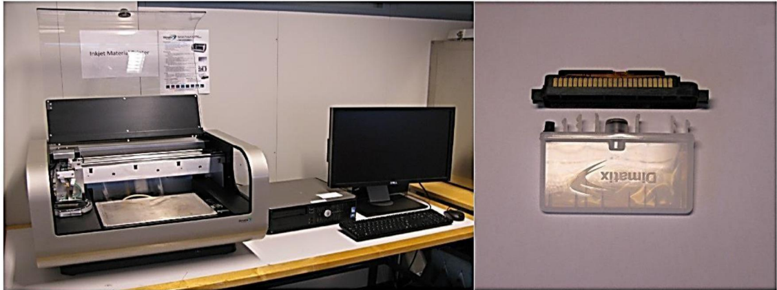
Figure 9. Dimatix DMP 2831 material inkjet printer and The cartridge and head used for printing.
