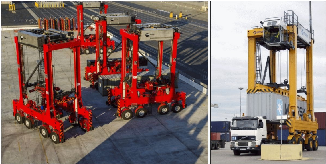
Figure 1.2 Automatic straddle carriers and manual straddle loading cargo. (Kalmar)
