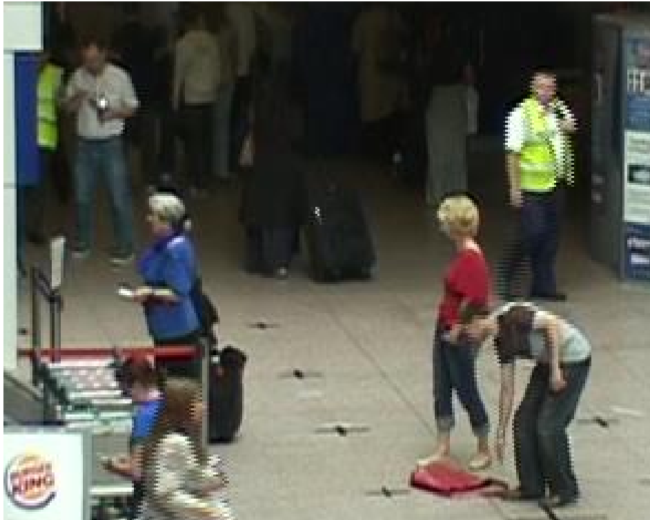
Figure 3.3: Separate fields causes edges of moving object to blur.
