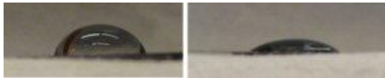
Figure 3.5: A barely hydrophobic Teflon® surface (left) and a very hydrophilic silicon nitride surface (right).
