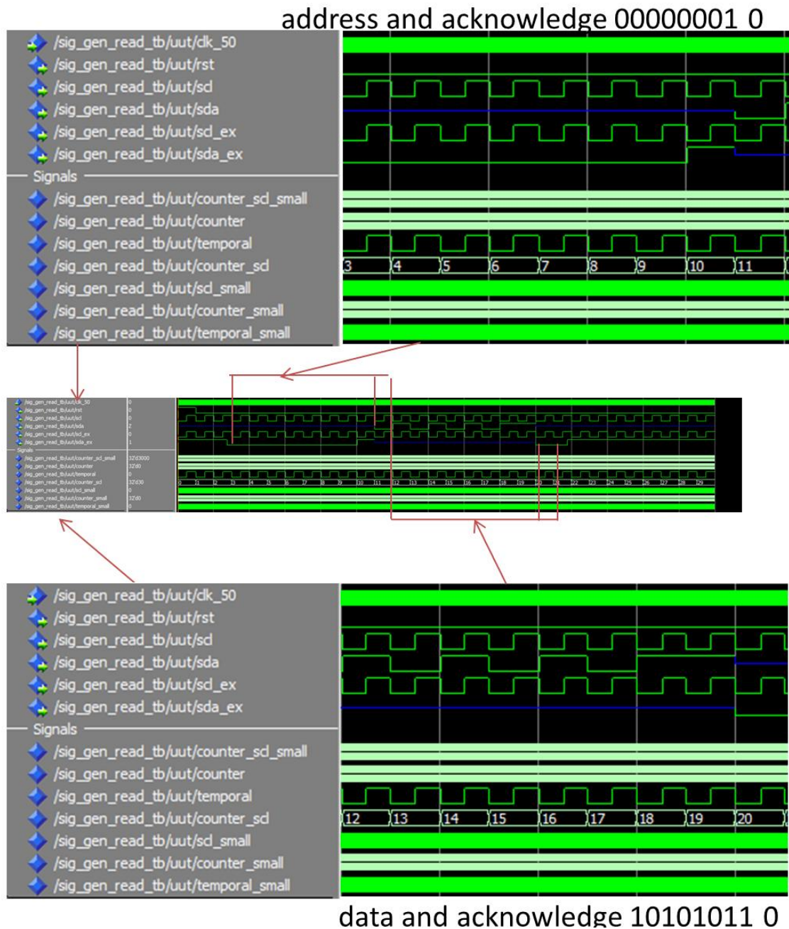
Figure 4.16 Modelsim testbench for address and data transmission of Signal Generator To Read in Reading Data Process.
