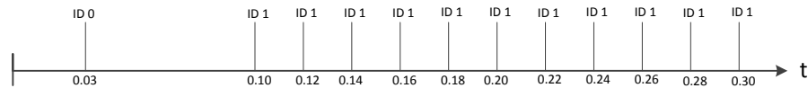
Figure 4.3: Example of describing two events. Event named input1 is executed once at 0.03 seconds from the beginning of the simulation. Event timer1 is executed repeatedly every 0.02 seconds starting from 0.1 seconds.
