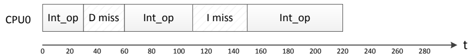
Figure 5.6: Example of a cache definition for processing element. Distributions used in the definition randomly chooses the amount of clock cycles to the next cache miss. That amount is generated again every time cache miss occurs. Timeline shows a task executing 160 integer operations on a PE cpu0 . The execution is stalled for 30 cycles due to data cache miss and 40 cycles for instruction cache miss, and thus taking 230 cycles to complete.
