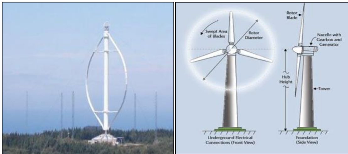
Figure 2.4 Two different types of wind turbine a) HAWT on left b) VAWT on right [12].
