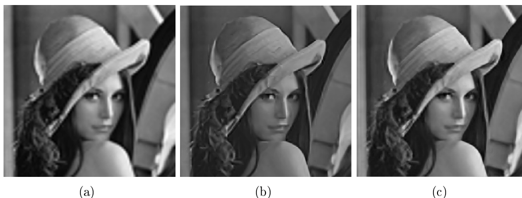
Figure 4.6: Lena image a) bicubic interpolation b) self-similarity, various patch size, small coefficients of ratio 3 c) self-similarity, direct ratio 3, various patch
