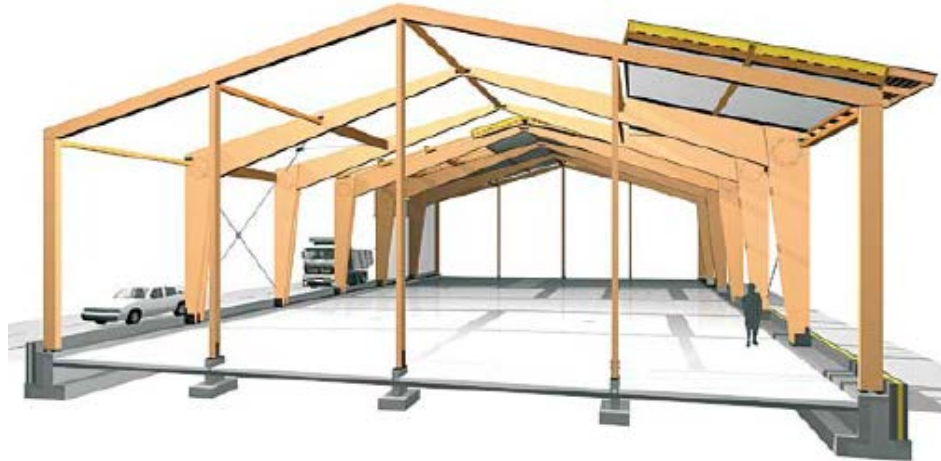
Figure 3.3 Portal frame for a single-storey hall building carried out with bolted or screwed haunches and braced with large roofing elements (Source: Puuinfo Oy 2009 p. 82)
