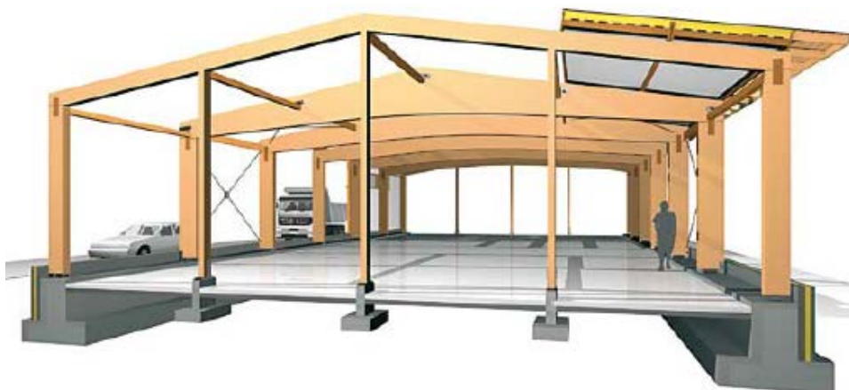
Figure 3.2 Mast frame for a single-storey hall building carried out with a boomerang beam and braced with large roofing elements (Source: Puuinfo Oy 2009 p. 74)
