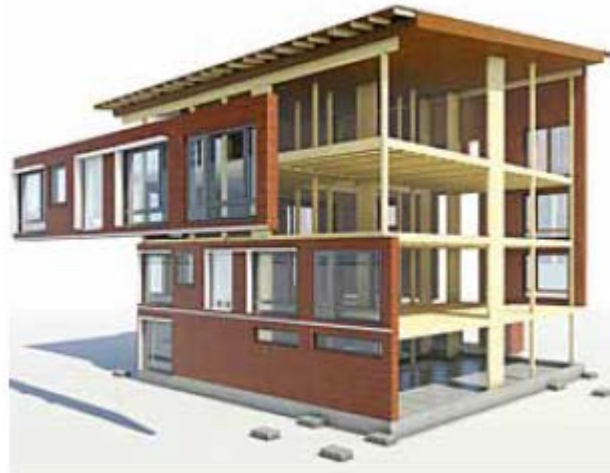
Figure 3.6 Beam-and-post frame multi-storey system in a combination with prefabricated building elements (Source: Metsä Wood 2013c)
