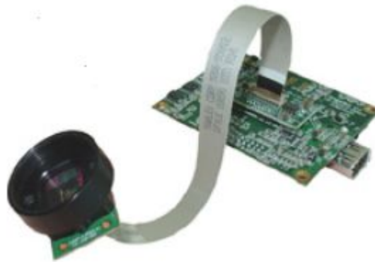
Figure 25. Dragonfly 2 camera with extended head [24]
