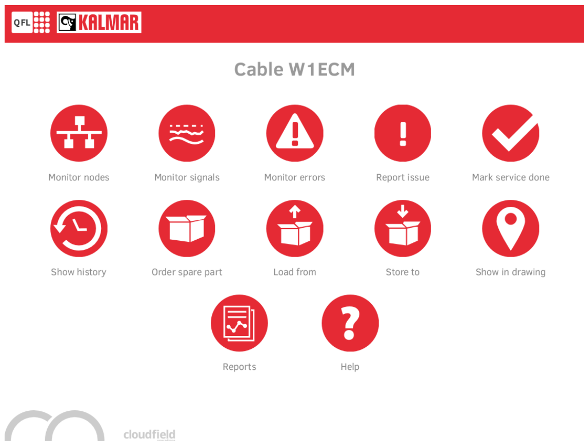
Figure 2.8 Screenshot of the QFL web application; service workers can, for example, report issues, order spare parts and view electrical drawings through the application.
