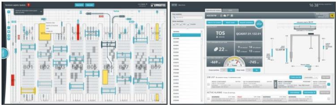
Figure 5.4 Screenshots from Fleetview. Fleetview shows the positioning of container handling equipment and active alarms in real time, and allows controlling the machines individually.
