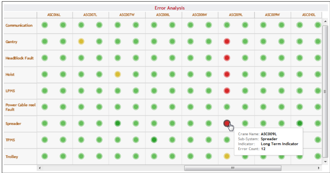
Figure 5.21 Crane ASC009L has had some errors related to Spreader.
