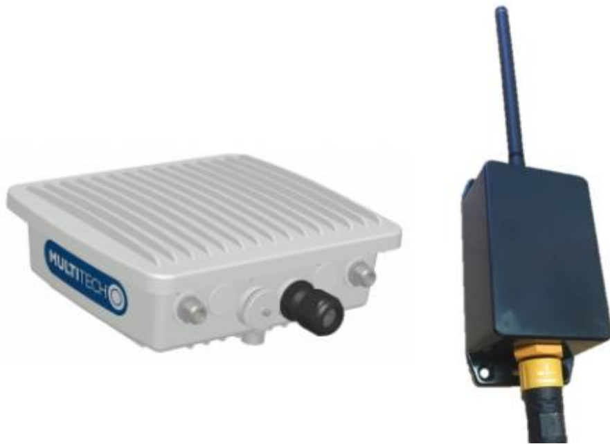
Figure 5.9 LoRa Gateway on the left and LoRa transmitter on the right. (Ala-Paavola 2016)
