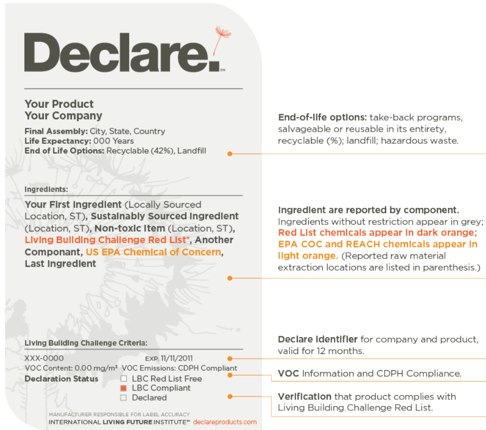
Figure 2.3 Declare label template and information about how and what transparency data is represented in a Declare label (ILFI 2018a).
