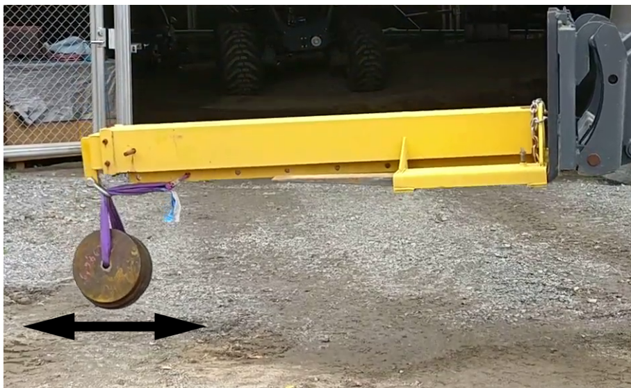
Figure 8.15. Load attached to the tip of the boom. Arrow indicates the added swinging direction due to fastening method.
