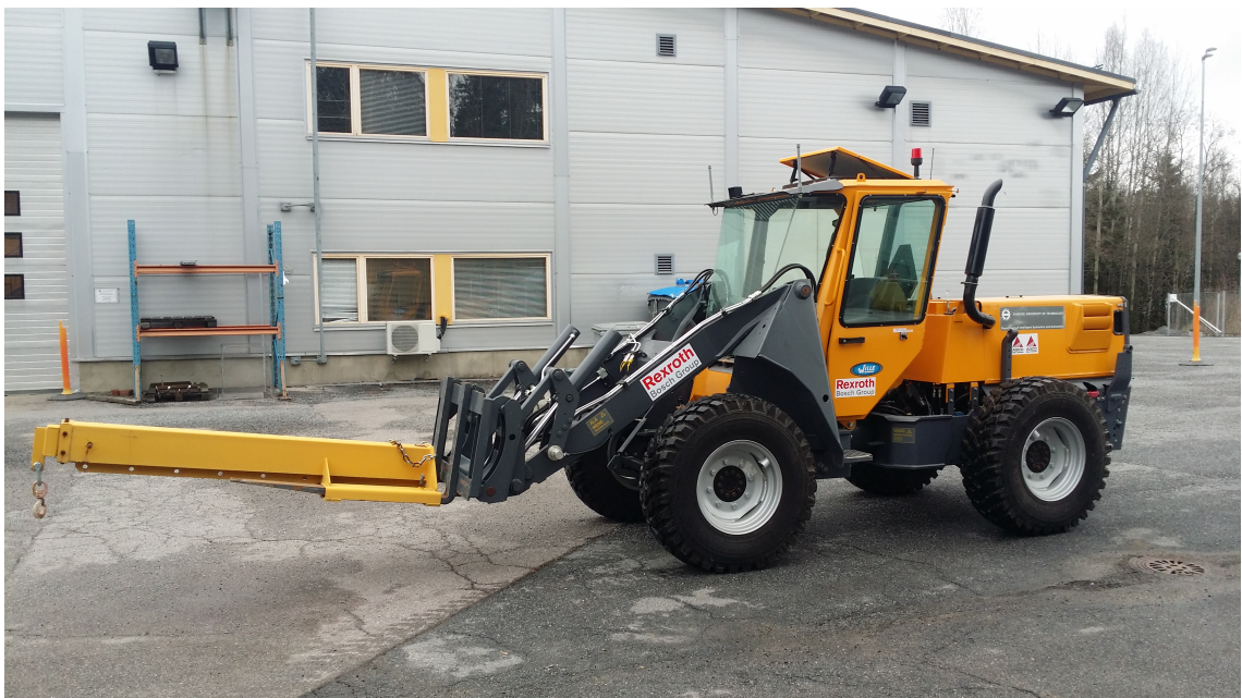
Figure 7.1. IHA-machine wheel loader with extended crane mounted to the tilt frame.
