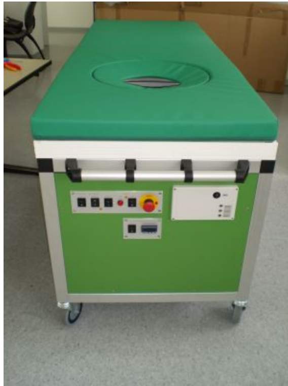
Figure 2.2 Examination table for 3D ultrasound computer tomography, source: Karlsruhe Institute of Technology
