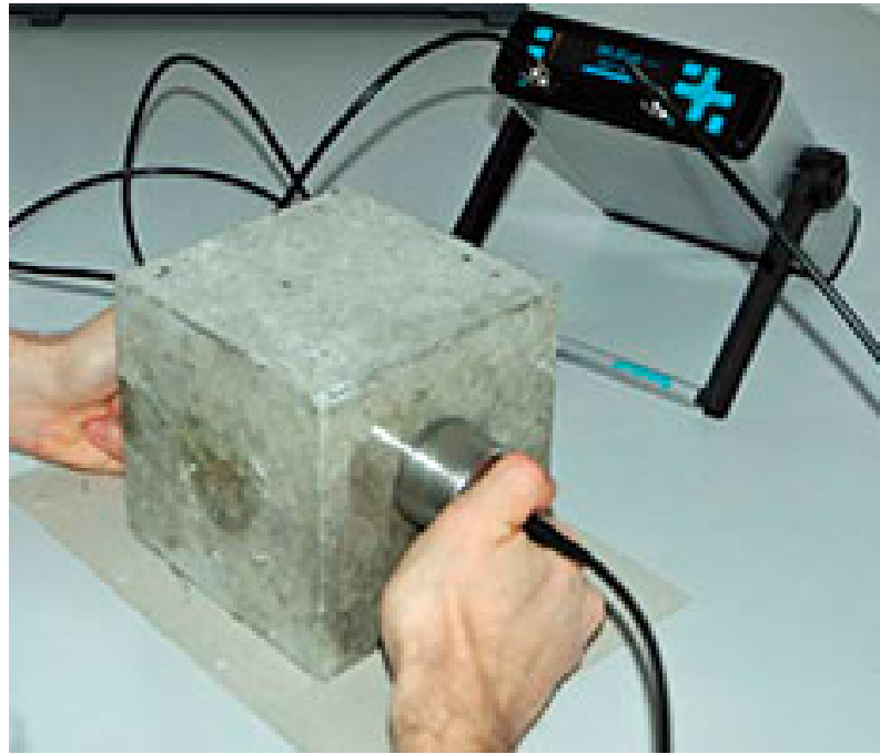
Figure 2.1 UPV testing of concrete using Pundit Plus, source: Germann Instruments
