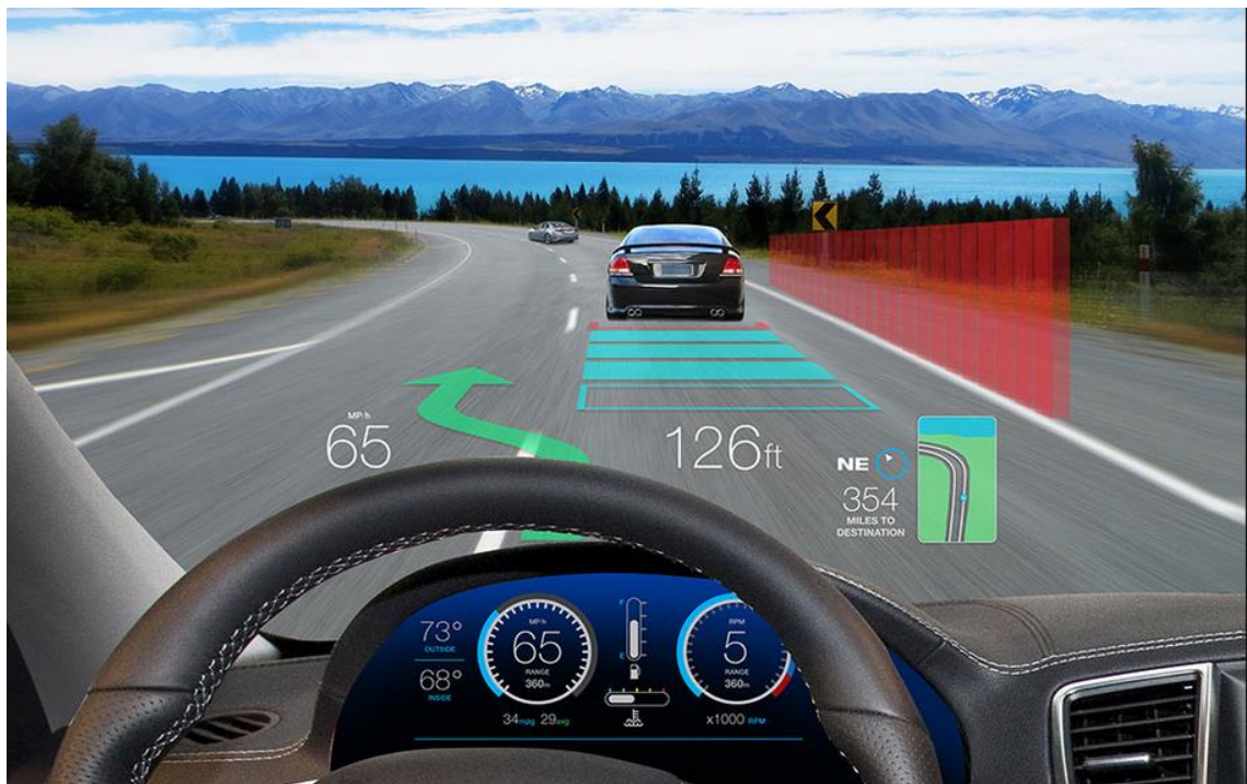
Figure 6 An augmented reality HUD and fully digital instrument cluster (Texas Instruments, 2016).
