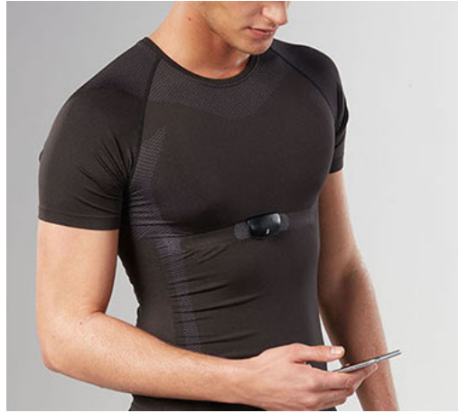
Figure 2.5 An example of wearable ECG monitoring system, integration of Clothing+ textile-integrated electronics (disappeared into fabrics for optimum comfort, durability and convenience) and Suunto wireless transmitter that transfers the recorded data to a smartphone app
