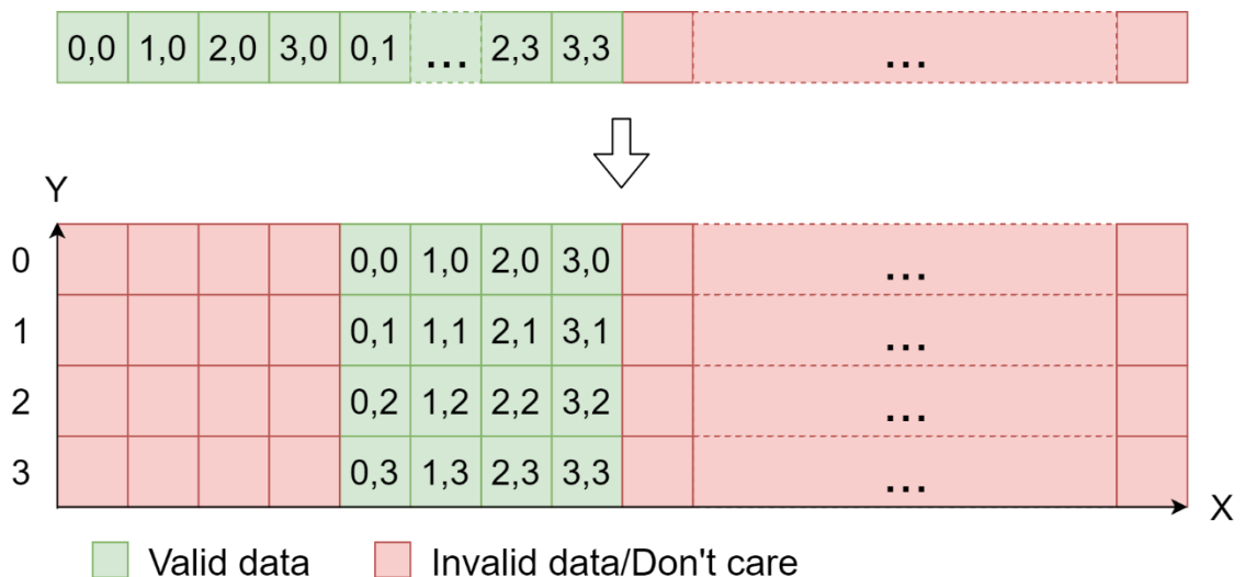
Figure 16. Slices to columns transform for 4 x 4 CB
