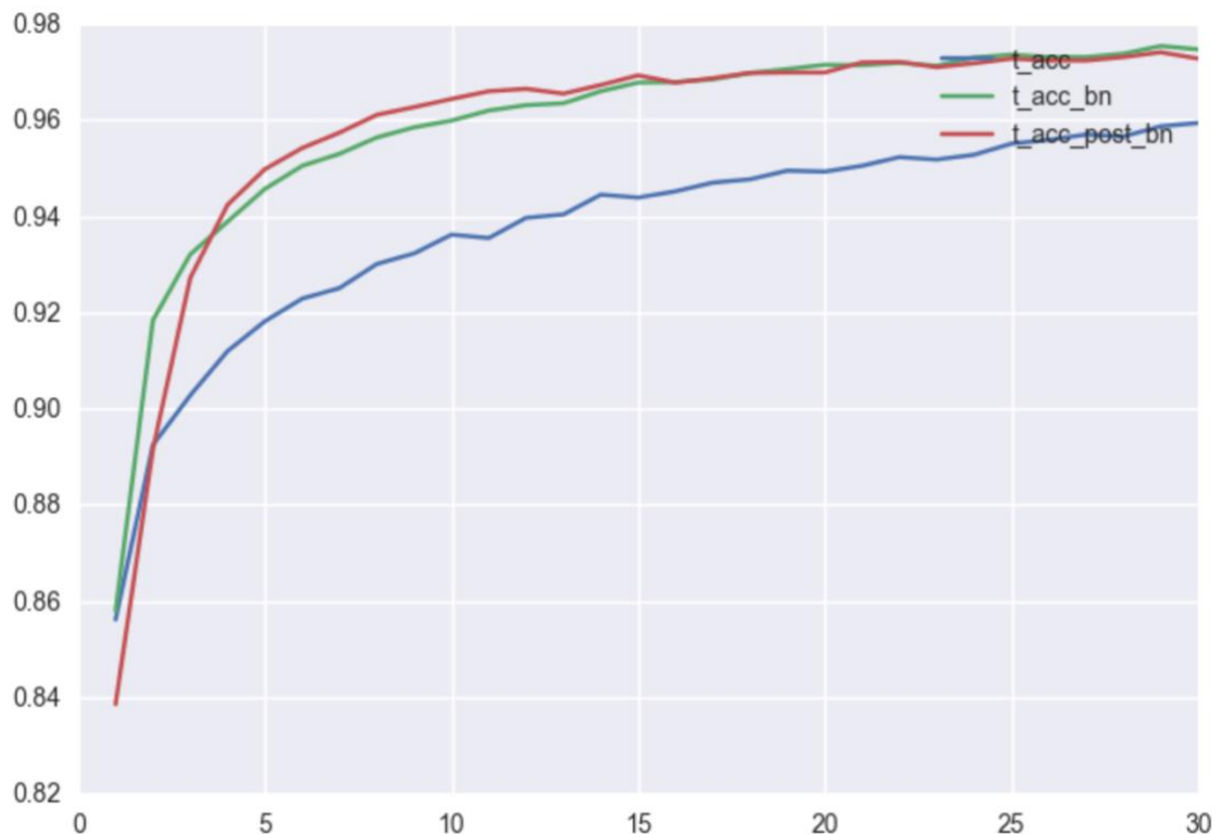
Figure 22 Performance with and without batch normalization
