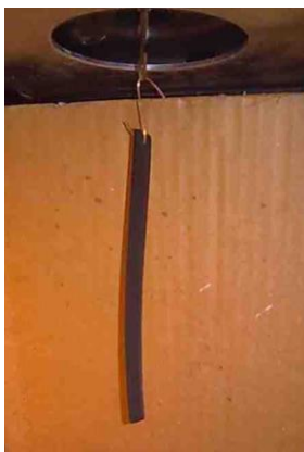
Figure 7.6. Weighing in air. Wire hook was attached to the sample and then the hook was attached to the hook of the balance in order to weigh the sample.
