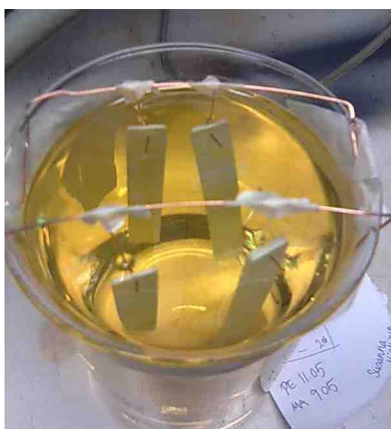
Figure 7.8. The samples were hung from the wire hooks and immersed in oil.
