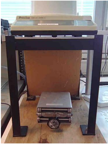
Figure 7.5 Precisa 500 M- 2000 C balance, which was used to measure the weight of the samples. The balance has a hook under it, so it was possible to weigh the samples.
