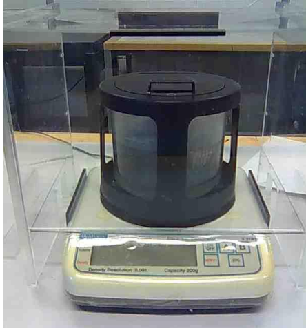
Figure 7.9. Wallace density measuring device used in these measurements. Weighing in air happened on top of the black container. Weighing in water happened inside the container.
