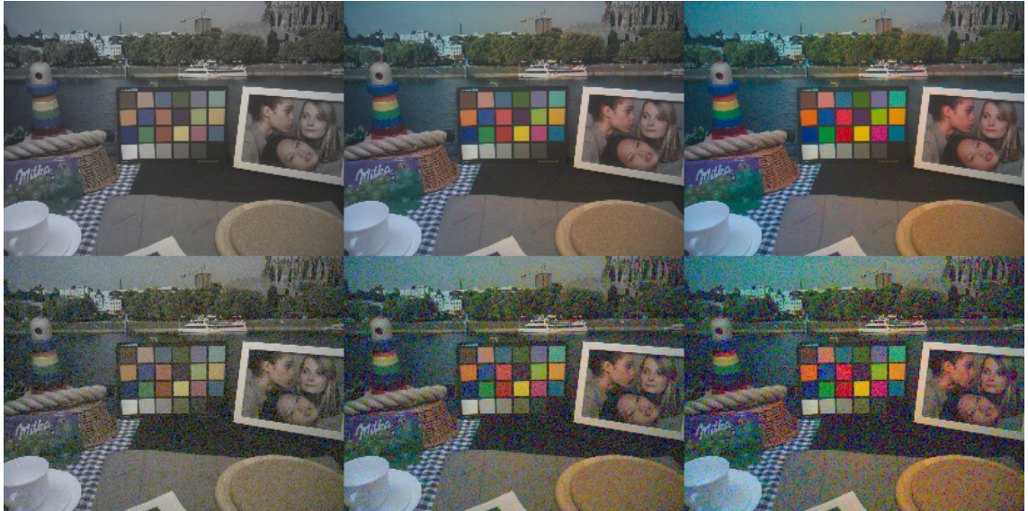
Figure 30 Output of white balance and color correction algorithms for noiseless and noisy images. In top row are noiseless images. In bottom row are images where Gaussian noise is added with noise variance 0.001. From left to right color correction multipliers are 0, 1 and 2.
