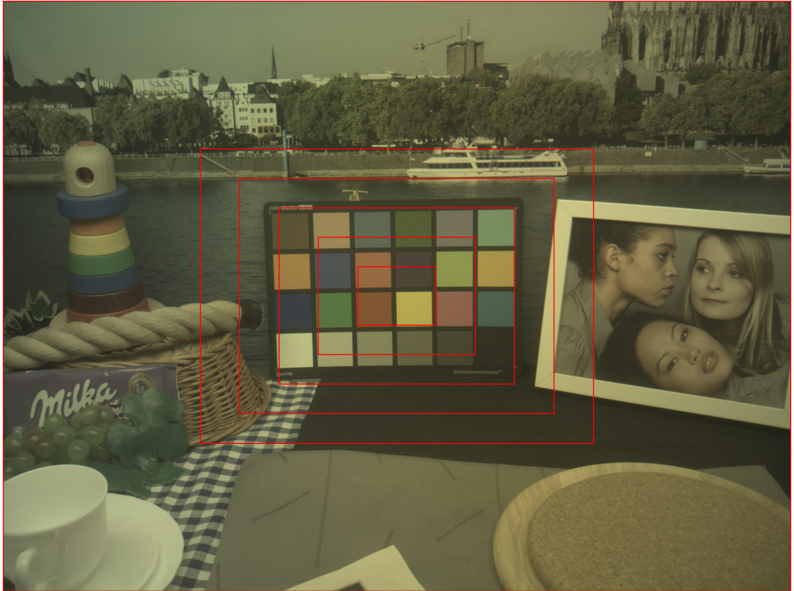
Figure 23 Image where different size of focus window sizes are presented. Window sizes are 10%, 20%, 30%, 40%, 50% and 100% of the full noiseless image.
