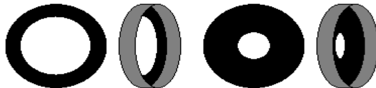
Figure 12 Here is presented very simplified version of camera lens system. It has only aperture and the opening where light comes into the system. Black color represents aperture and gray color inner borders of camera lens system. This figure consists of 4 images. From left to right 1 st and 3 rd image are seen in front of camera, whereas 2 nd and 4 th image are seen from certain angle. In 1 st and 3 rd image only aperture is visible. In 2 nd and 4 th image the rightmost ellipse is the opening and inner white area is aperture corresponding to 1 st and 3 rd image.
