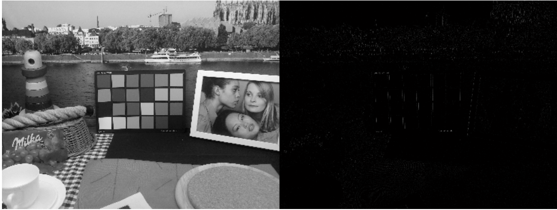
Figure 34 Example of filtering image with high pass filter of order 6 presented in figure 32.
