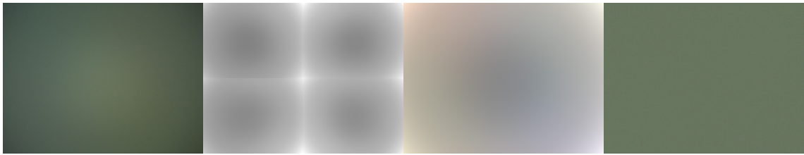
Figure 14 Here is presented vignetting correction. From left to right first is presented unprocessed image. Next are show 4 smaller gray scale images, which are corresponding vignetting correction for each color component (Gr, R, B and Gb). Next is shown overall combined effect of these color components. In last image vignetting has been corrected.
