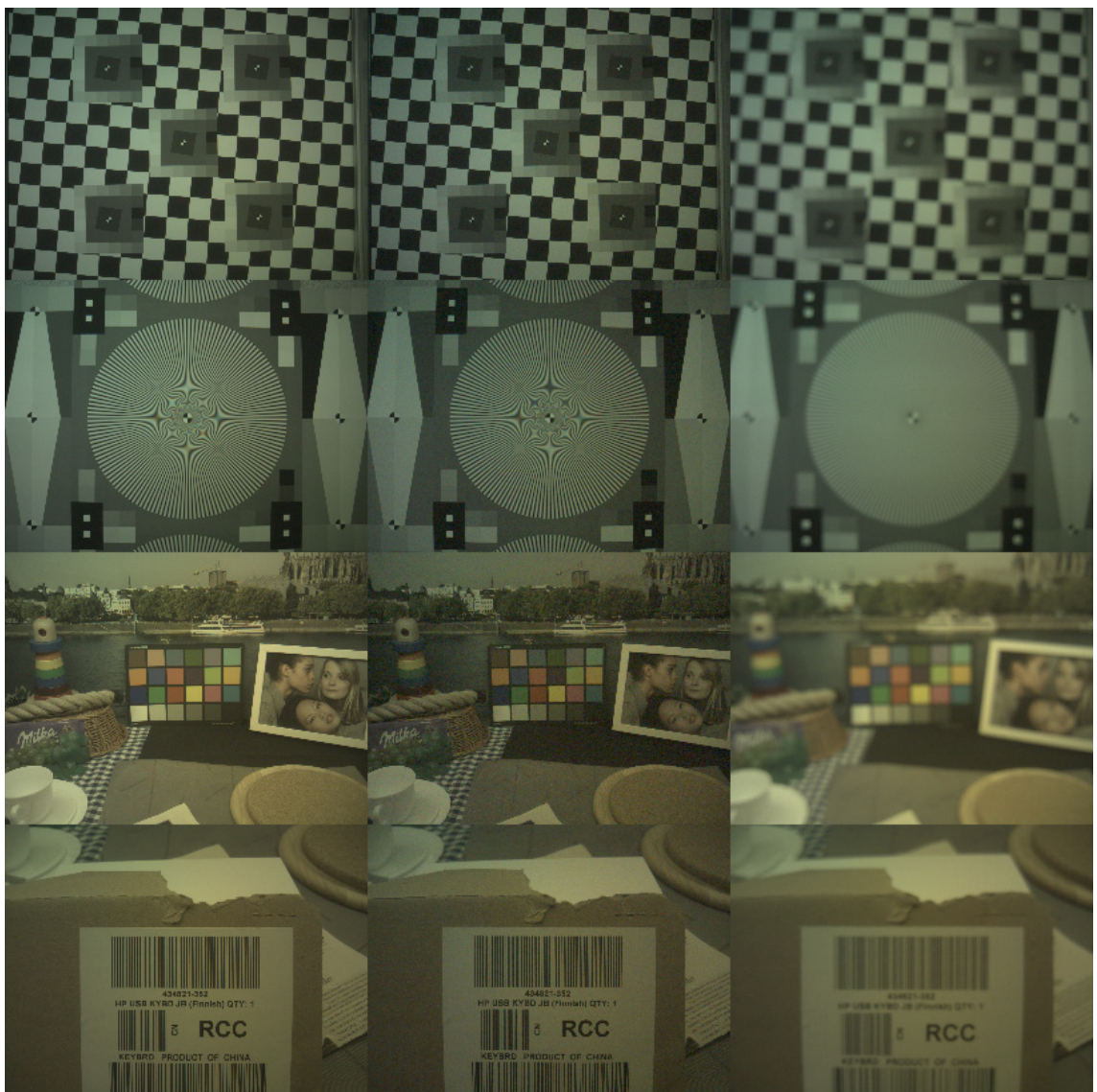
Figure 19 From top to bottom downscaled images of scenes AF box, Siemens star, light studio and barcode. From left to right are presented in-focus image in high illumination, in-focus image in low illumination and out-of-focus image in high illumination. Later in this thesis images in first column are called noiseless.
