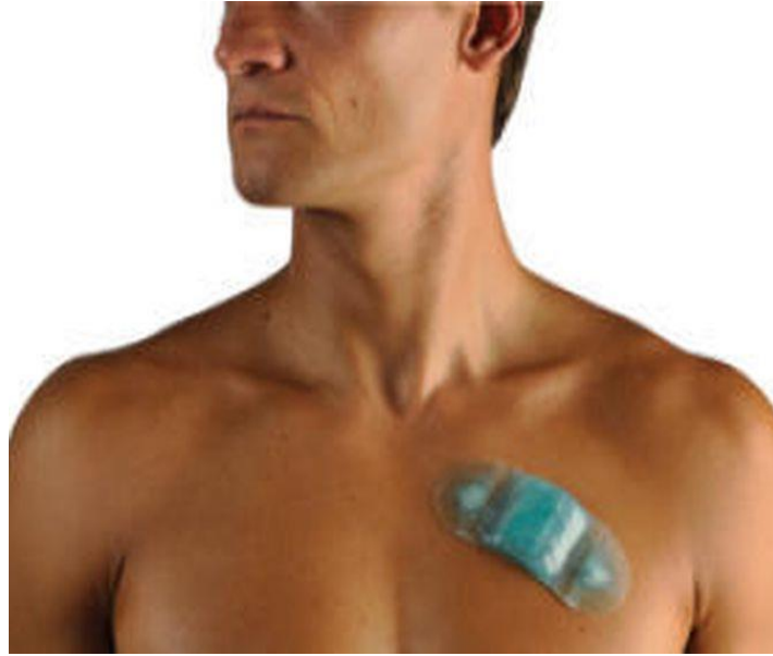
Figure 12. The placement and orientation of Zio Patch Module [47].
