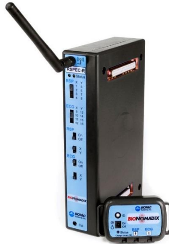
Figure 22. BN-RSPEC Transmitter and Receiver Module [59].
