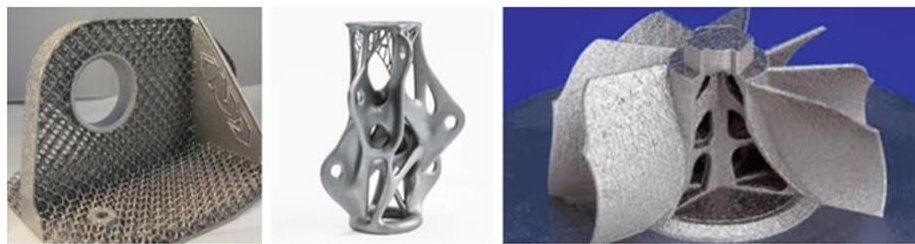
Figure 15. Some freeform AM parts that are difficult to inspect[11]
