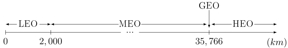
Figure 2.1: Altitudes of Low (LEO), Medium (MEO), and High Earth (HEO) orbital zones, and the geostationary orbit (GEO). The zero-level is Mean Sea-Level (MSL).
