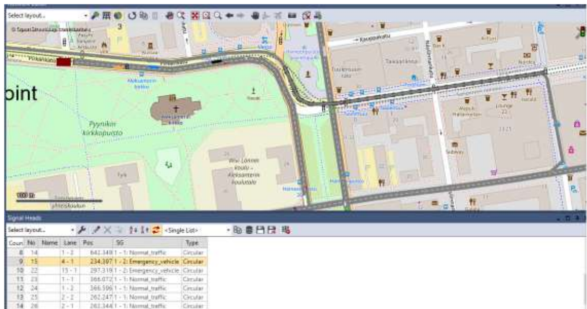
Figure 22: Different traffic signals in network
