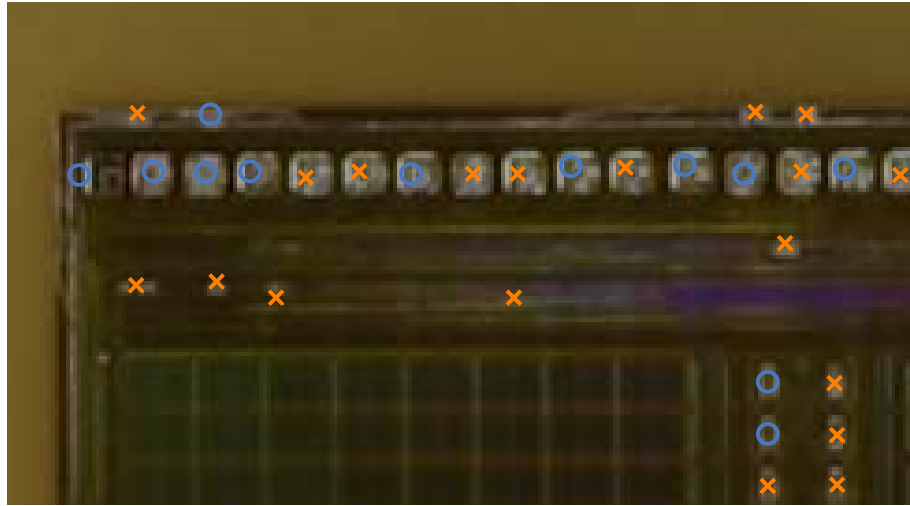
Figure 5.4: Connection point detection results of the upper left corner of the third IC on module number five. Blue circles indicate the positive classifications and orange crosses indicate the negative classifications.
