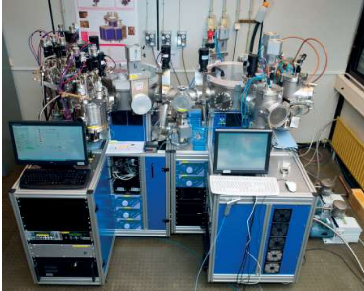
Figure 1. The overview of the CT1000 cluster deposition tools (van den Hurk 2016)
