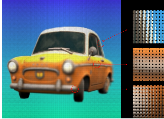
Figure 3.14 Sensor image of the defocused plenoptic camera, where the scene depth range is 0.4\text{m} - 0.6\text{m} (Slava Z. ©2014 www.sketchfab.com, used under the Creative Commons Attribution license).
