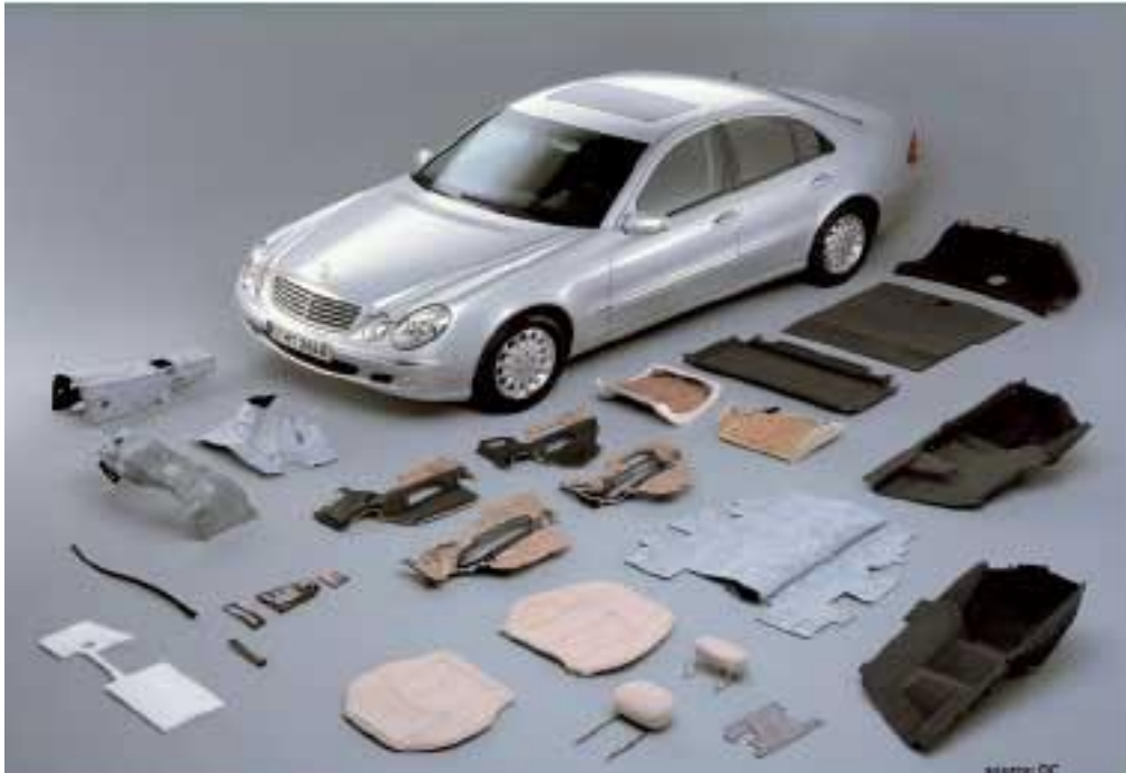
Figure 20: Natural fiber composites in a Mercedes E-Class [51].
