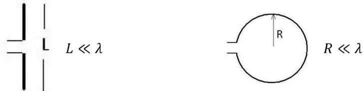
**Fig. 3.5** Examples of electrically small antennas small dipole (left) and small loop (right)
