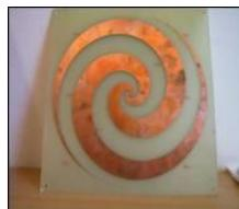
**Fig 3.7** Spiral antenna as an example of broadband antenna. [61]
