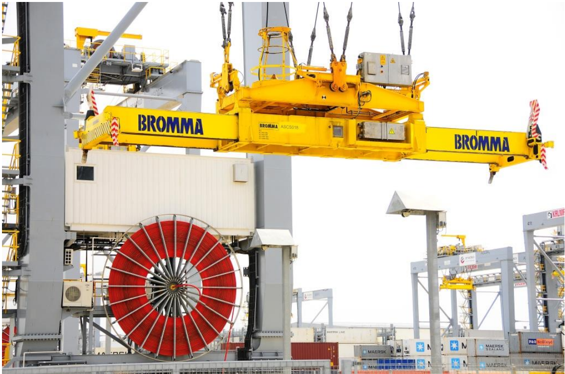
Figure 5: Close-up view of a spreader, with ASC cranes in background [9]
