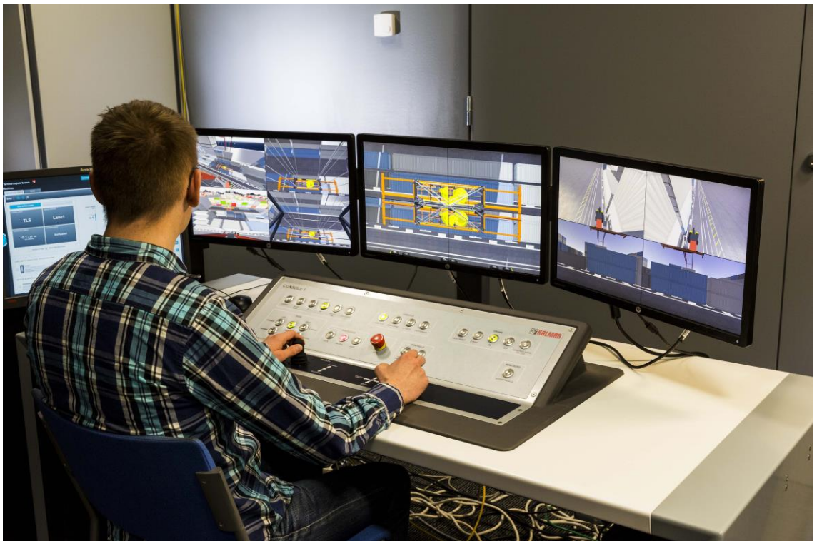
Figure 12: Operating of an RTG simulator via a remote control table [23]
