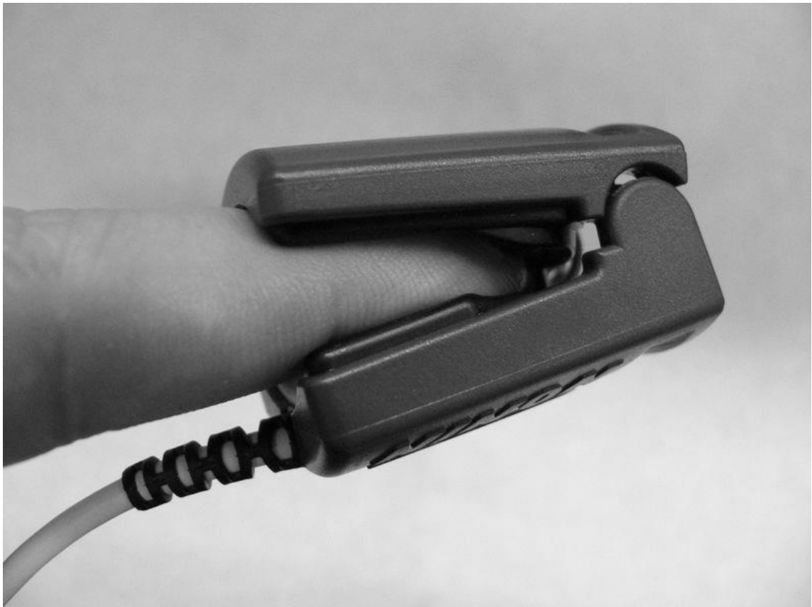
Figure 5. A blood oxygen saturation meter using transmission mode of PPG (Rama, 2005)
