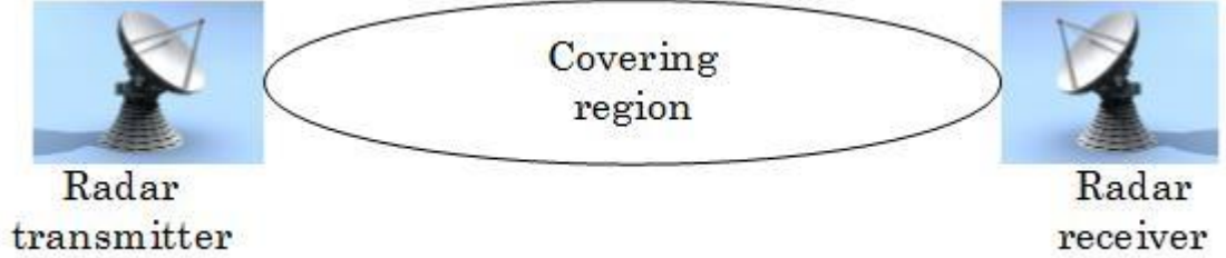
Figure 2.3: Simple illustration of bistatic radar
