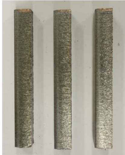
Figure 83: 6 mm copper's cutting edges. From the left to right upper, middle and lower part of the edge.
