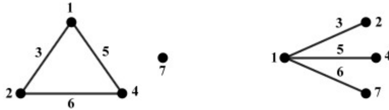
Figure 38: Two linear graphs for L8 matrix adapted from [37]
