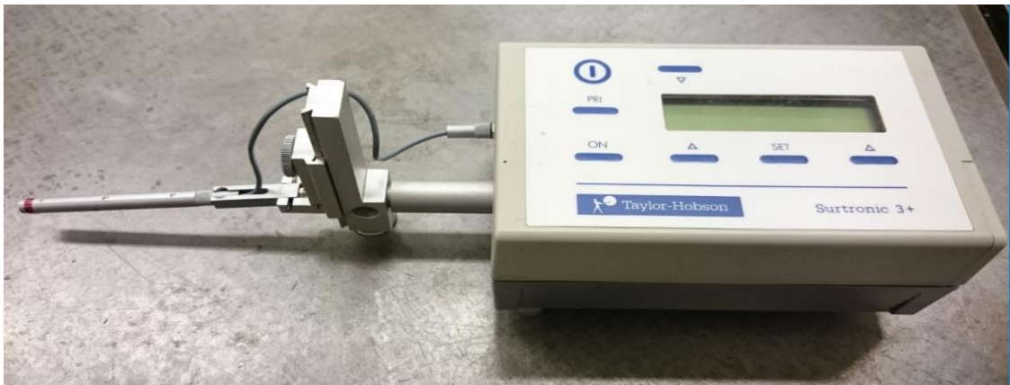
Figure 43: Taylor - Hobson Surtronic 3+ surface roughness measurement tool. [47]
