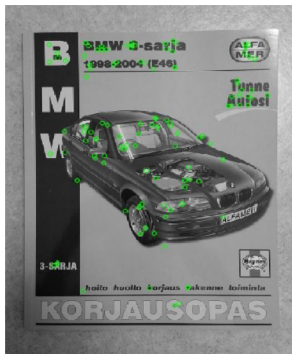
Figure 2.1: Keypoints in the image, shown as green circles.
