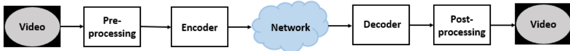
Figure 4.4 Block diagram of the encoding and decoding process of intra-frame coding methods
