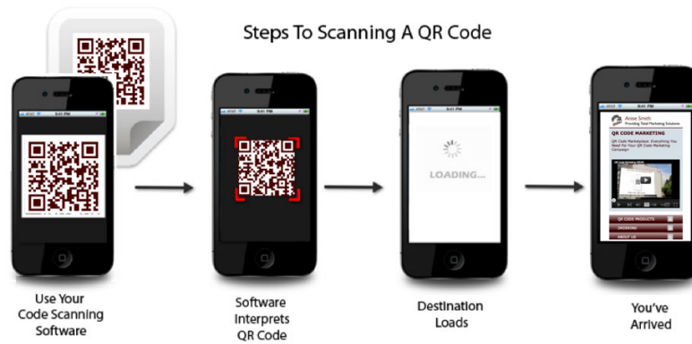
Figure 2.5 How the QR code system work [25].
