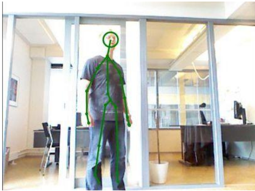
Figure 3.10. Turning the camera left, the right shoulder is 0.2 m closer to the camera than the left shoulder. Camera starts turning left with the speed of 15 degrees in a second.
