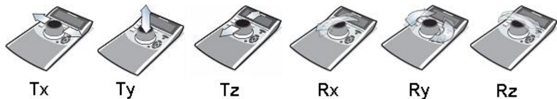
Figure 2.23. Cap functions of SpacePilot PRO: Cap can be both translated and rotated in 3 dimensions. [80]
