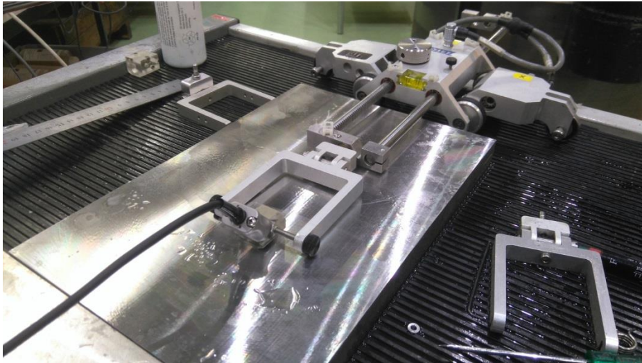
Figure 41 Scanner with a linear phased array probe attached and the specimen
