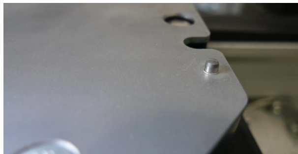
Figure 35. Positioning pin in detail
