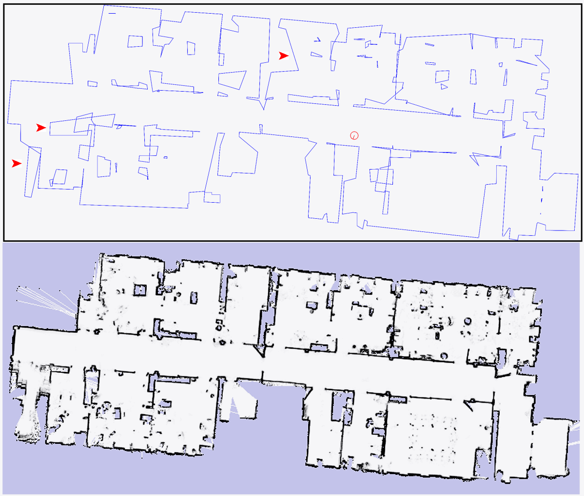
Figure 6.8: The Kalman filters method's result: After 1400 time steps. It is comparable with the map provided by occupancy grid mapping. The major errors are noted by the red arrows.
