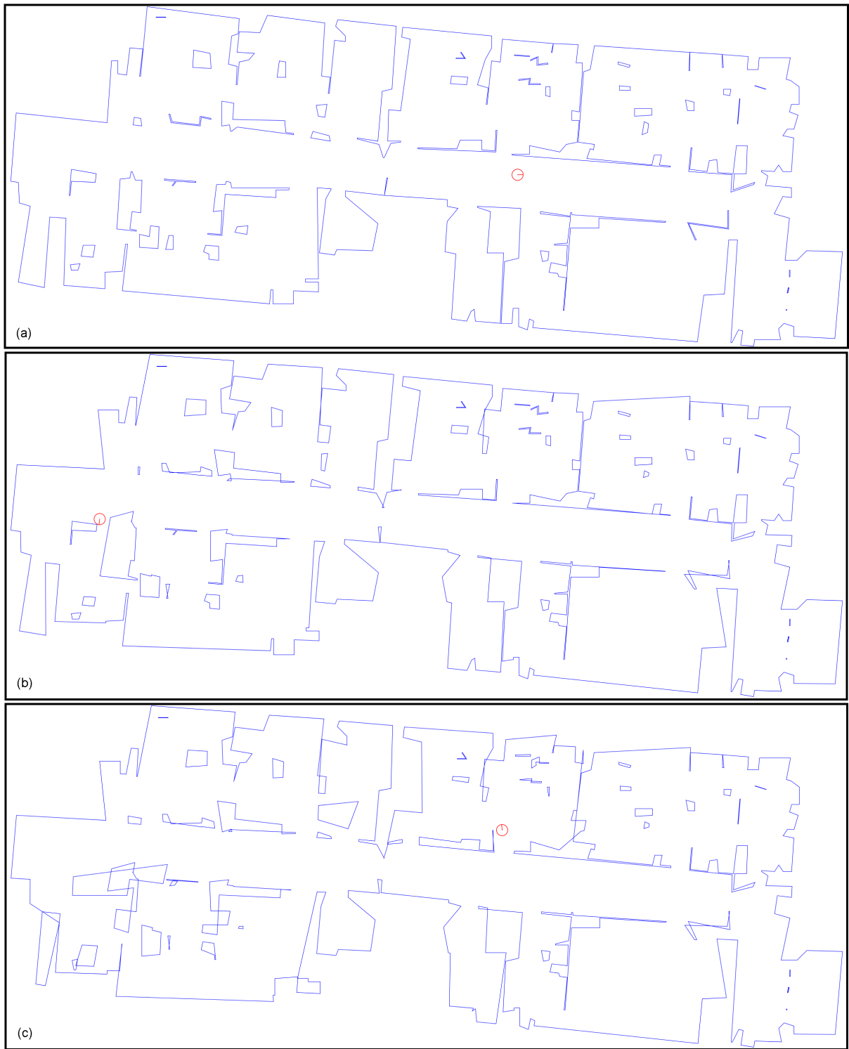
Figure 6.7: The Kalman filter update in progress: a) 1 st time-step. b) 340 th time-step. c) 760 th time-step.
