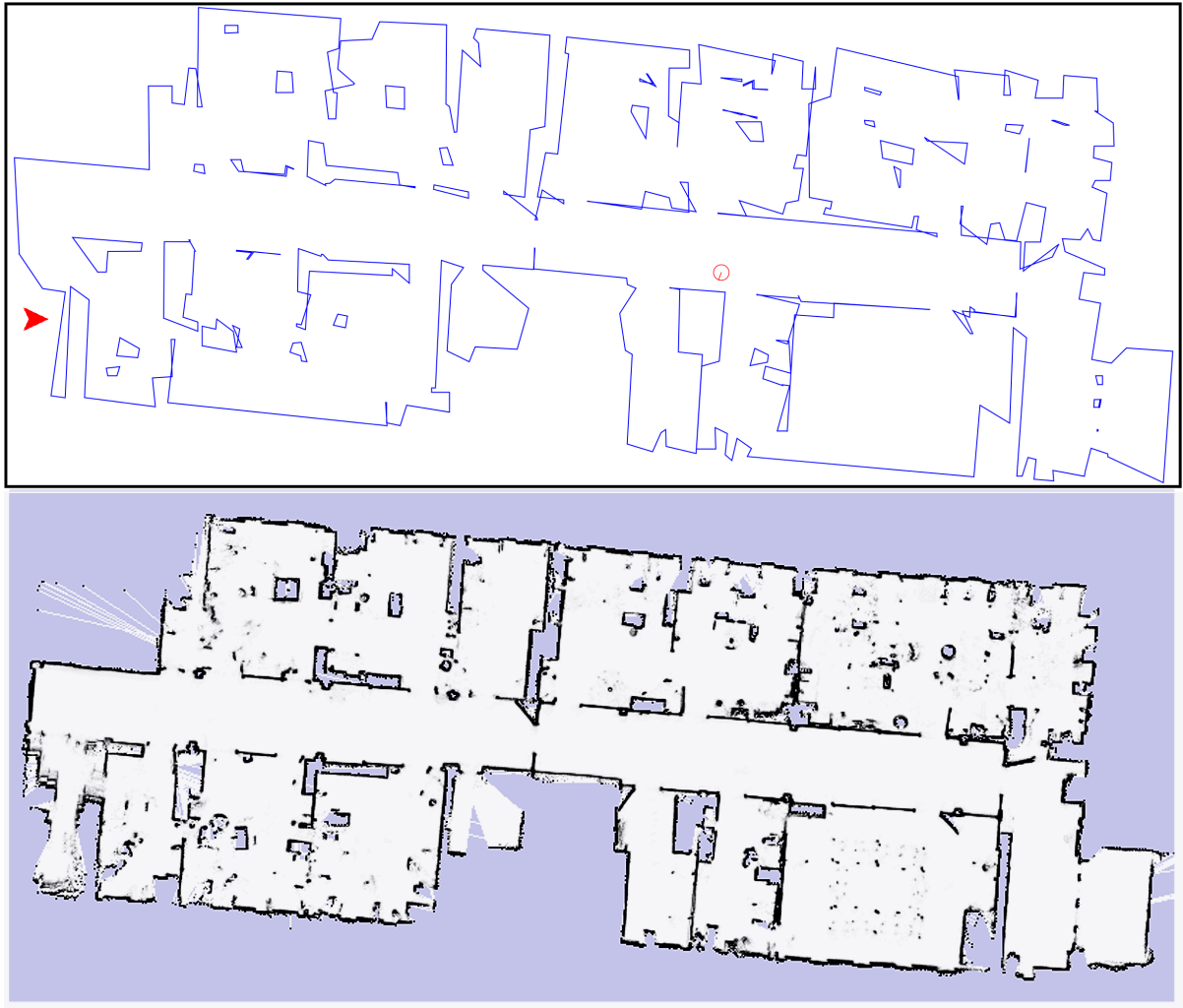
Figure 6.12: Geometrical constraint method's result: After 1400 time steps. It is comparable with the map provided by occupancy grid mapping. The major errors are noted by the red arrows.
