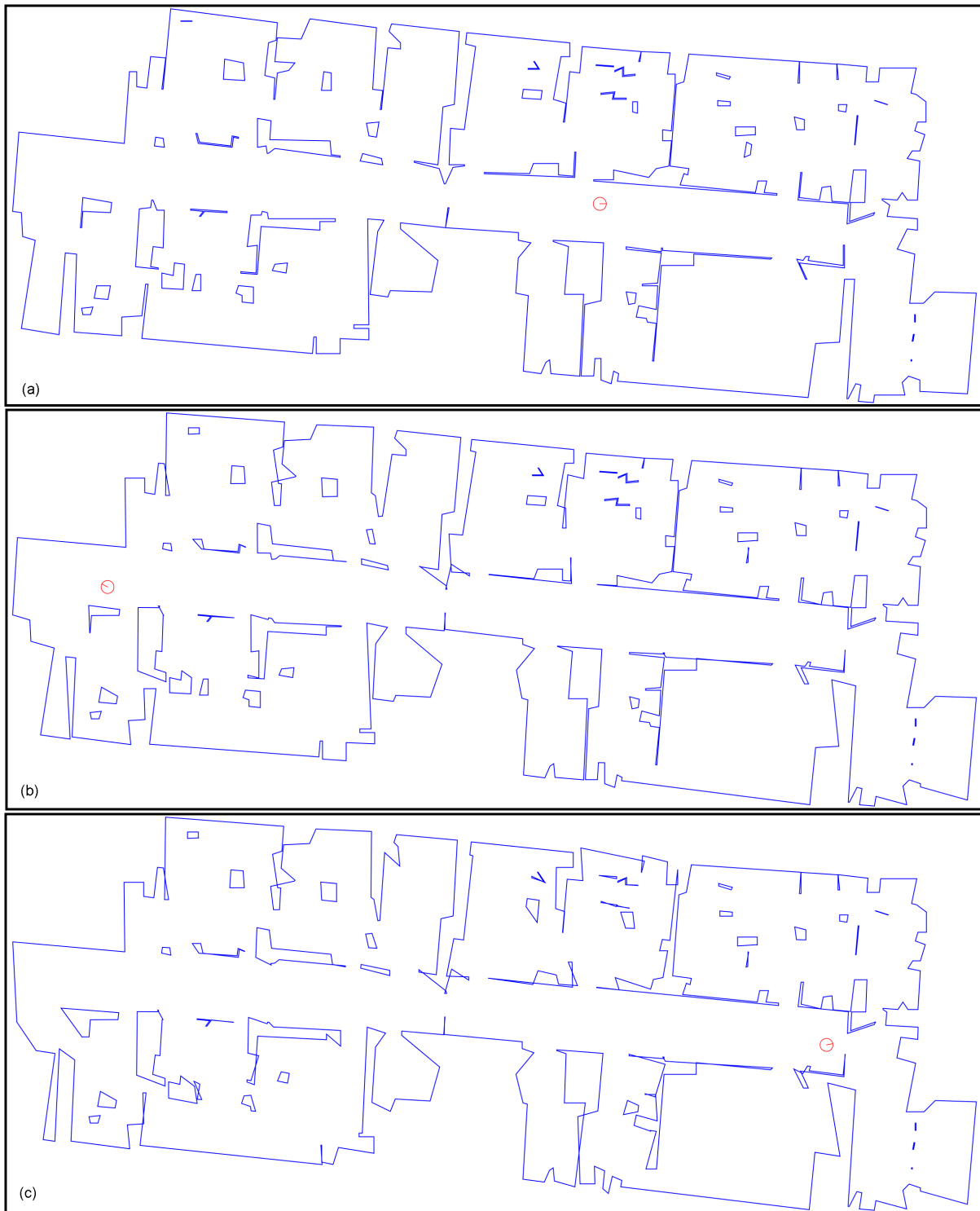
Figure 6.11: Constraints update in progress: a) The prior map at 1 st step. b) The map after 380 th time step. b) The map after 913 th time step.
