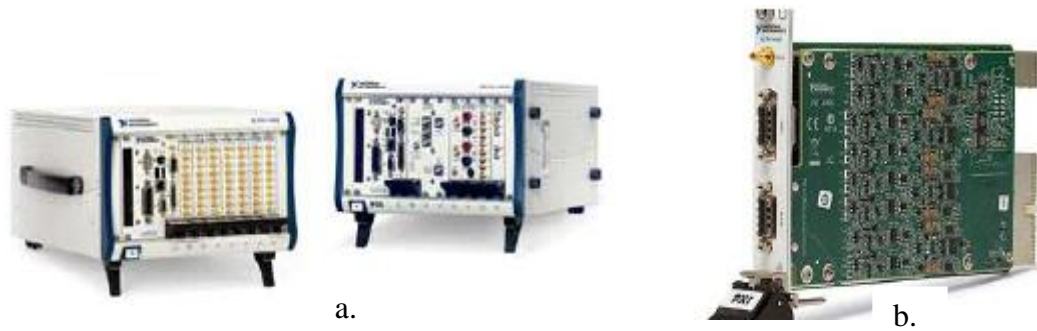
Figura 42 Hardware de National Instruments a. PXI-1042Q b. PXI-4496 (Instruments, s.f.)
