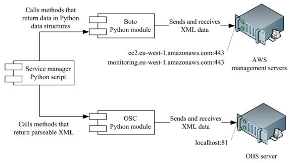
Figure 4.4. Script components and their connections
