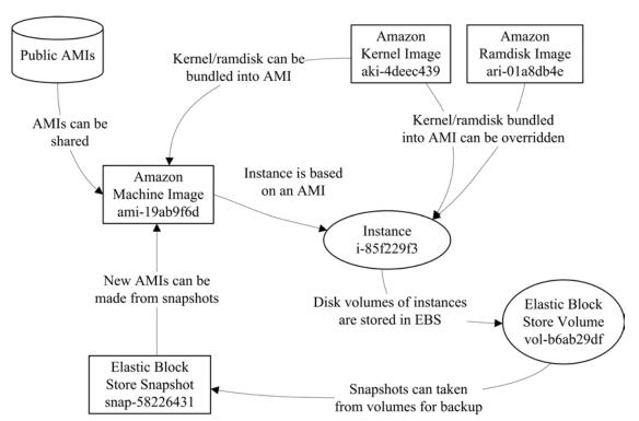
Figure 4.3. EC2 instances are created from Amazon Machine Images
