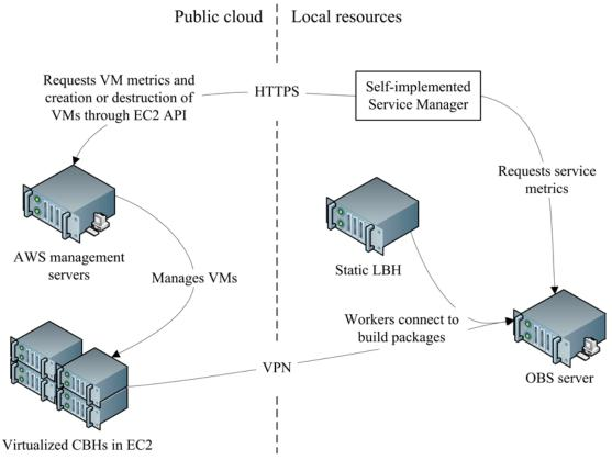
Figure 4.2. Simplified architecture implemented in this work
