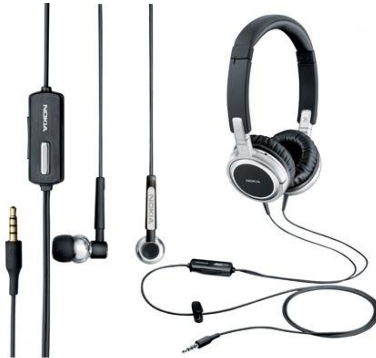
Figure 2.6. Two headsets with a microphone, an earpiece and an answer/end call button [1]
