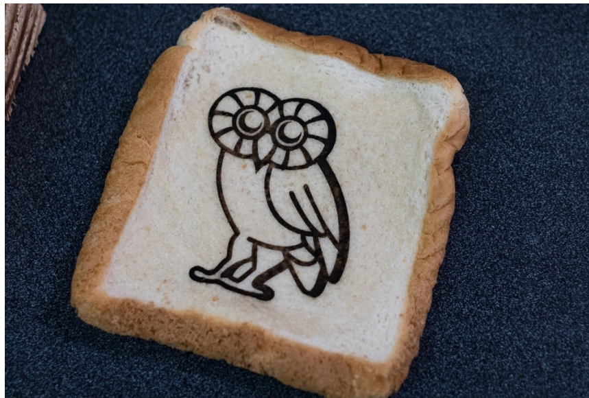
Figure 4.2: Edible toast etched with laser-induced graphene [82]
