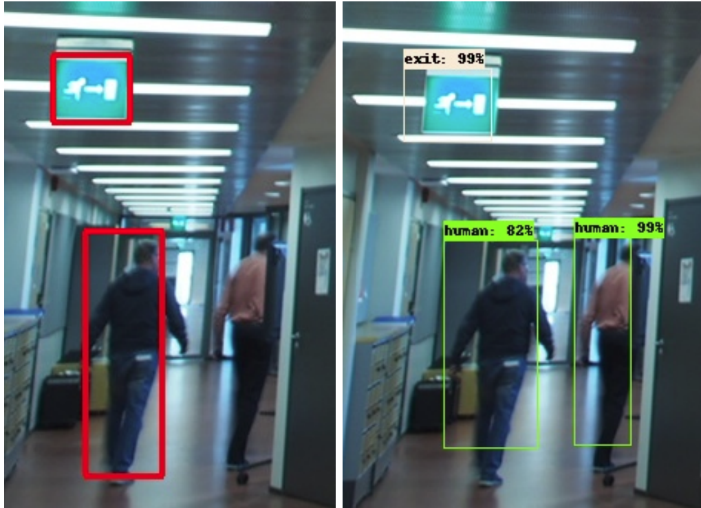
Figure 5.4 The left image contains two annotated objects: a human and an exit sign. The right image is resulting image of the detector. It found two humans and an exit sign.
