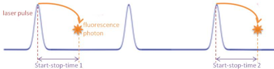
Figure 8. Measurement principle of start-stop times in time-resolved fluorescence measurement with TCSPC, diagram adapted from (Wahl 2014a).
