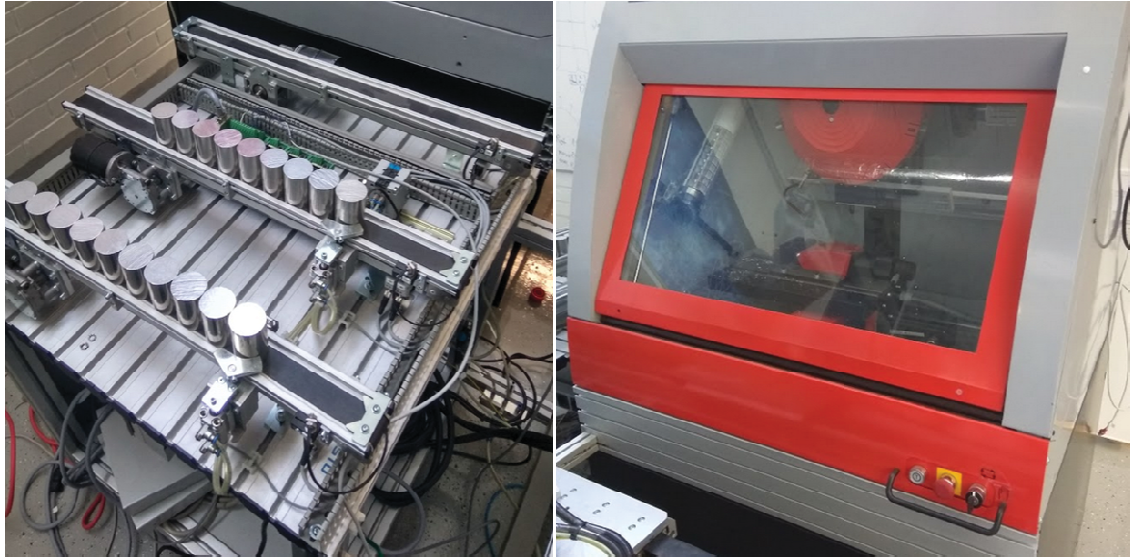
Figure 20. Buffer station (left) and CNC machine (right)
