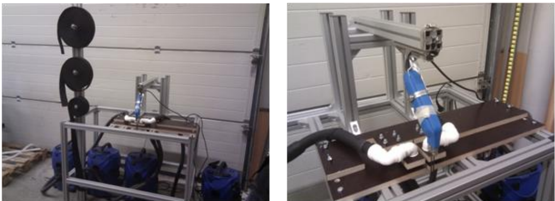
Figure 72. Continues sleeve cutting with vacuum mechanism second version.
