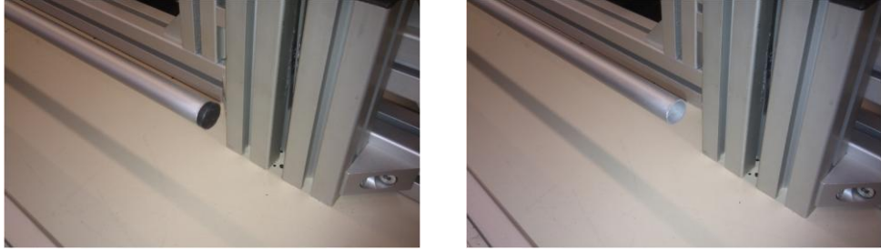
Figure 102. Removing plastic cap covering end of the aluminum tube.
