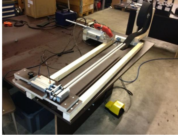
Figure 83. Assembling foot pedal and sleeve roll holder to the mock-up.
