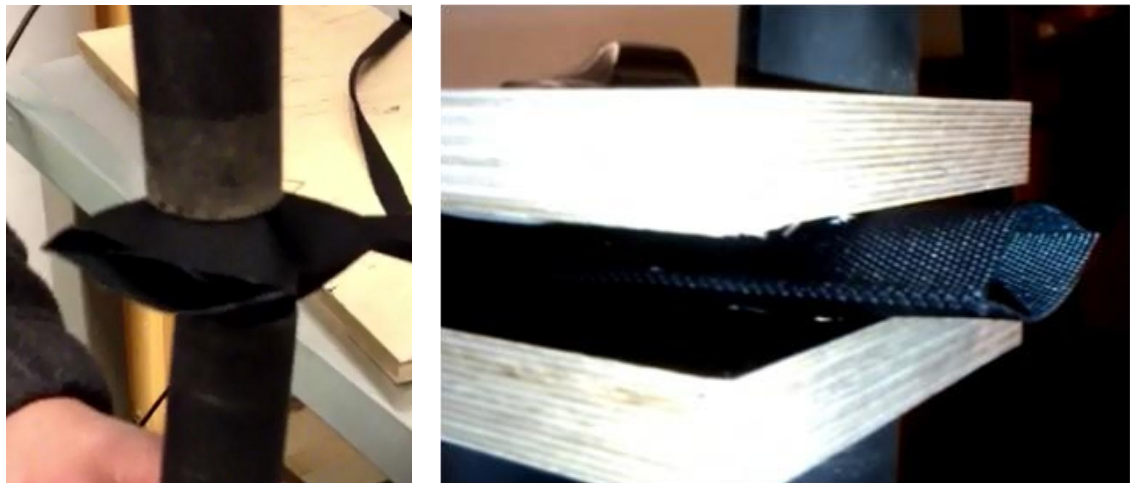
Figure 70. Vacuum mechanism utilization for opening sleeve sides.
