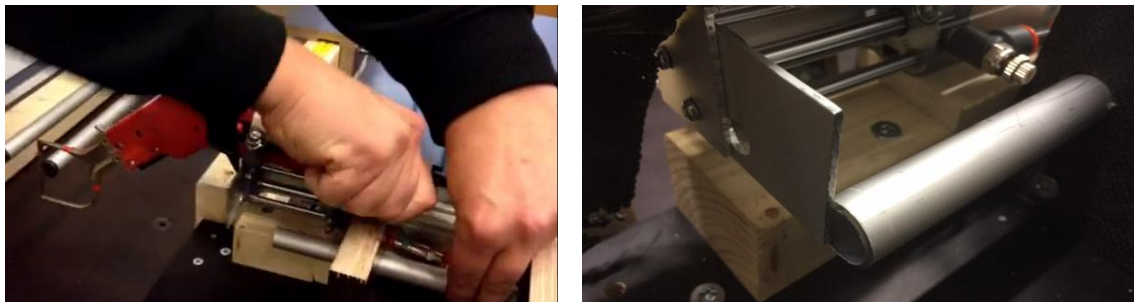
Figure 84. Backstop for controlling cylinder stroke.
