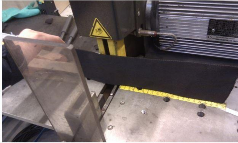
Figure 57. Preparing sleeve pieces with manual hose cutting machine.
