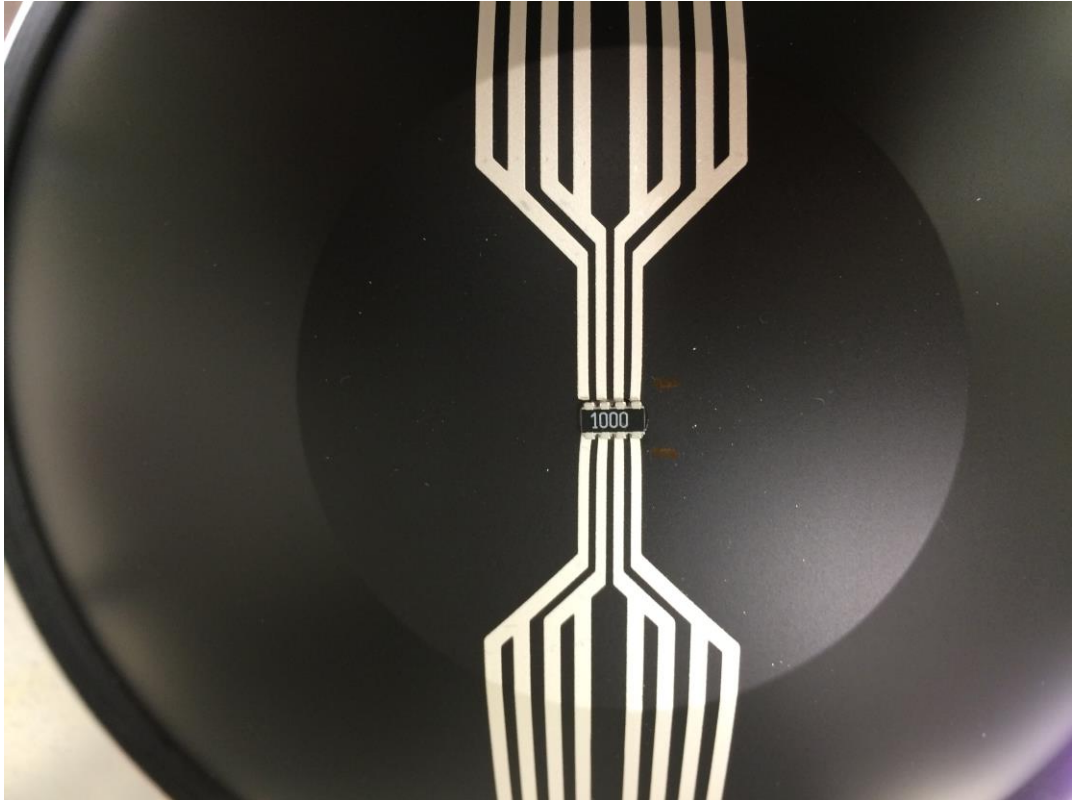
Figure 39. The breakdown of the adhesive joints under strain in custom-made test setup
