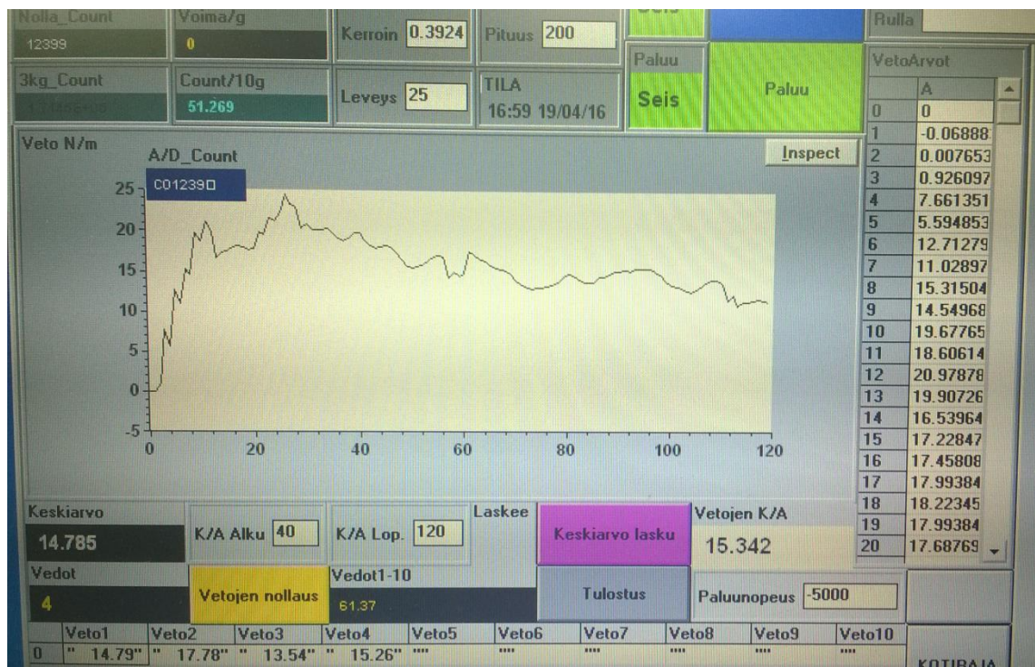
Figure 41. Example of a peel test curve. The final result is average value of the peel force at x-axis range 40–120 mm. Width of the sample is 25 mm and the result is given in units N/m.
